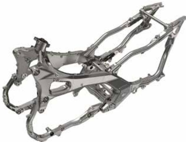
■ Robotically welded aluminum twin-spar frame with revised plate thicknesses in frame spars for optimized rigidity and flex characteristics. (Frame and swingarm are 4.4 pounds lighter.)
