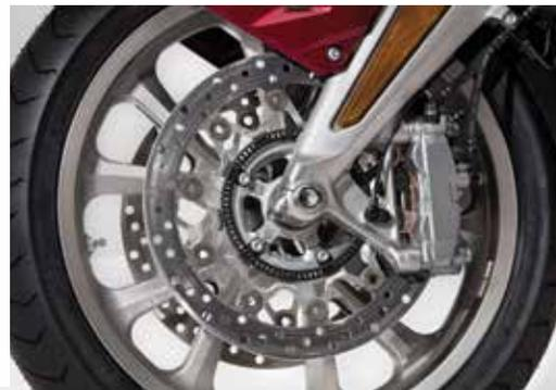
■ Electronically controlled combined ABS system with single modulator for reduced weight, and radially mounted 6-piston dual front-brake calipers.
