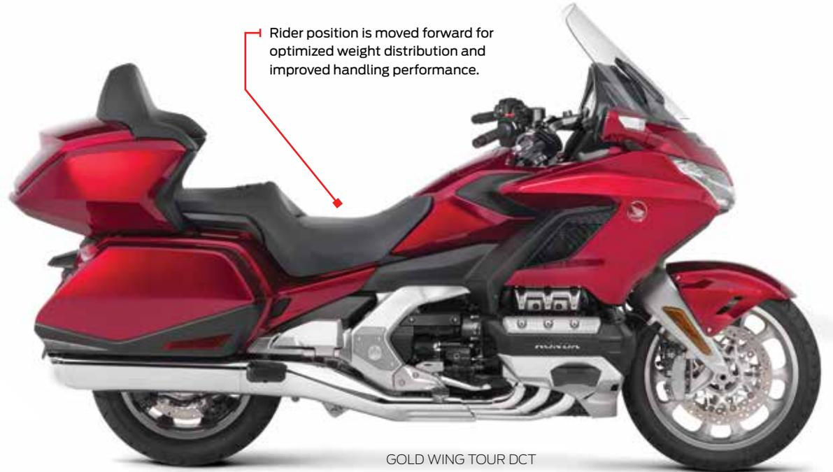
Rider position is moved forward for optimized weight distribution and improved handling performance.
